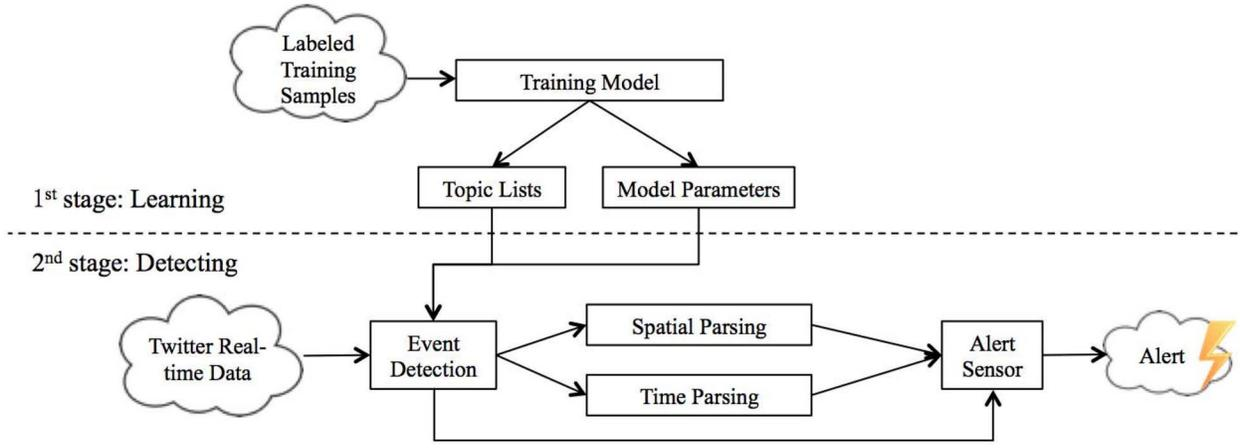
Fig. 3. Proposed framework for two-stage power outage event detection.
