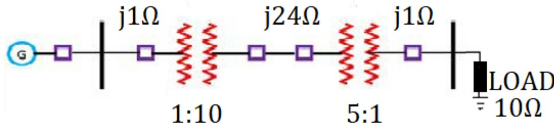
$$V_{B1} = 13.8 \text{ kV}, V_{B2} = 138 \text{ kV} \text{ and } V_{B3} = 27.6 \text{ kV}$$
