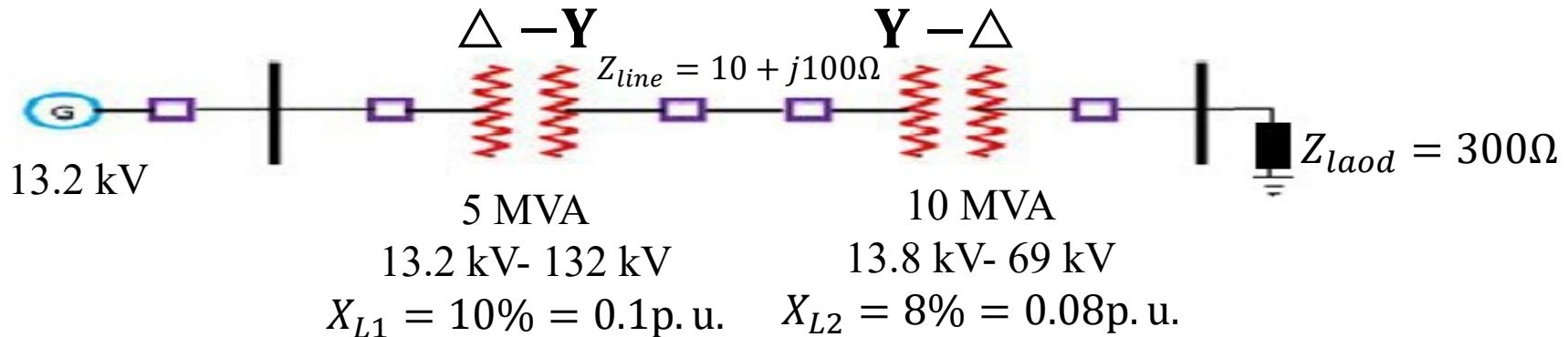
$$Z_{load} = \frac{350\Omega}{476\Omega} = 0.63 \text{ p.u.}$$
